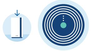
When the status LED is green, you are connected. The next three LEDs are indicating the signal strength.
