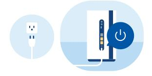
Plug in the power adaptor and then connect it to your gateway. Push the on/off button, the LEDs on the top of the gateway will turn on. Your Nokia Gateway will start to search for the best connection.
